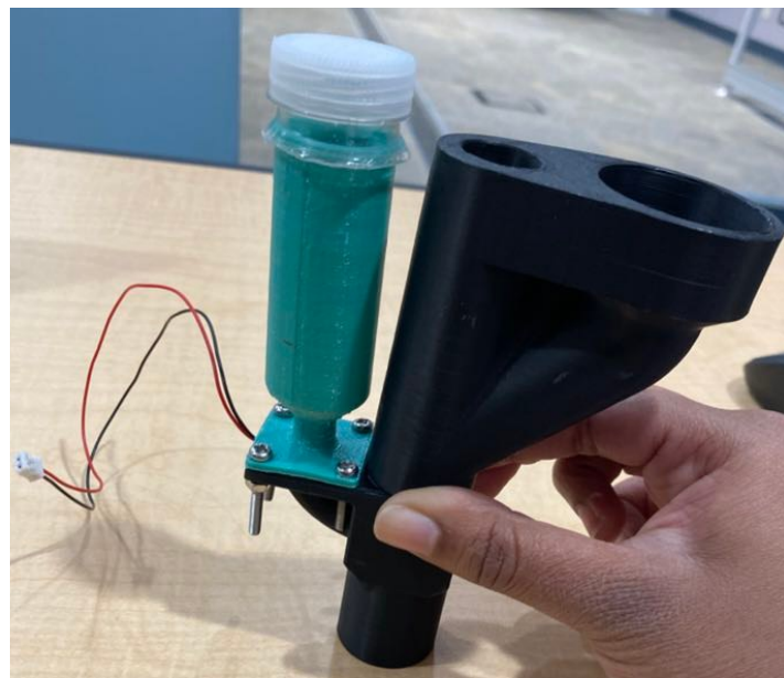
Figure 21. The Water Tank, Humidifier, and Mixing Chamber
