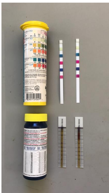
Figure 8. Test strips from ocean testing (inlet on left, outlet on right)
