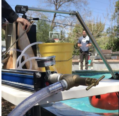
Figure 5. View of outlet tubing to show flowrate through system
