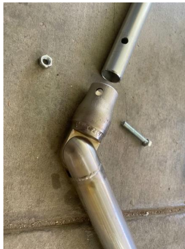
Figure 2. Lever arm to pump handle connection
