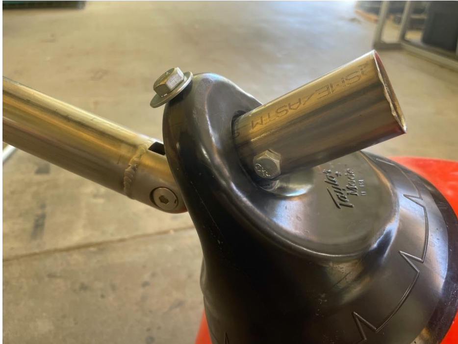
Figure 3. Buoy to lever arm connection
