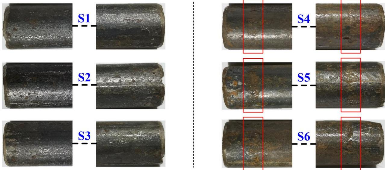
Figure 3. Corrosion of steel bar ends in each specimen
