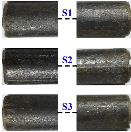
Figure 3. Corrosion of steel bar ends in each specimen
