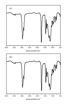
Figure 3. FT-IR spectra of (a) silicone-acrylic emulsion and (b) organic-inorganic hybrid super-hydrophobic coating
