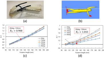
Fig. 1: Developed paddle and simulation results, (a) developed paddle (for the right arm), (b) simulation model, (c) dependency of  $R_T$  (ordinate) on forearm length (abscissa) and angle (legends) for crawl stroke, (d) dependency for backstroke.
