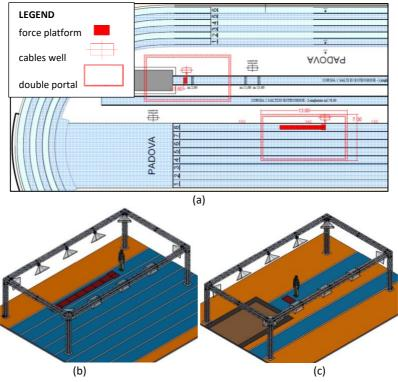
Fig. 1: Instrumented athletics track. (a) overall plan view, (b) detail view of the sprint track, (b) detail view of the long jump track.
