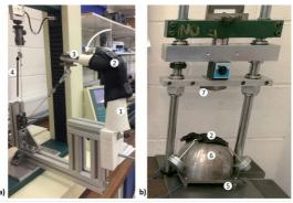
Fig. 1: ISO 20320:2020 performance test setups (a) limitation of wrist extension test (b) impact performance test. 1- Polyamide hand and wrist surrogate, 2 -wrist protector, 3 - steel rods to apply the load, 4 - displacement to generate torque in surrogate wrist, 5 - load cells, 6 - hemispherical dome, 7 - guided falling mass
