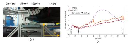
Fig. c: (a) Experiment setup installed in the TrakTester; (b) Relative movement of the tip of the stud in relation to the shoe sole postition
