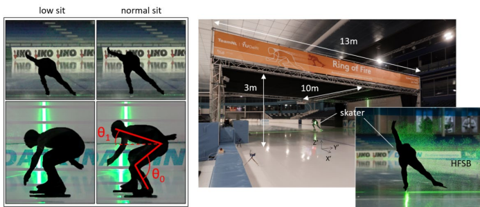
Figure 1: front and side view of the two skating postures (left) and the experimental arrangement (right).
