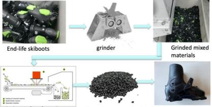
Tribolectric/NIR/metal sorting Secondary raw material New skiboot Fig. 1: scheme of the process for recycling of ski-boots
