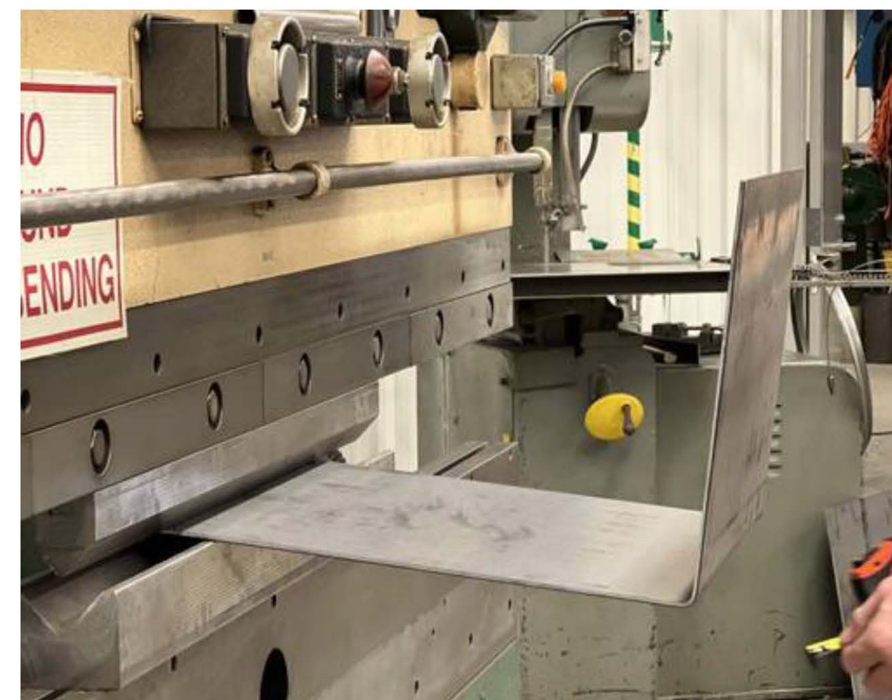
Figure 7. Bend thick materials if necessary for the preferred design
