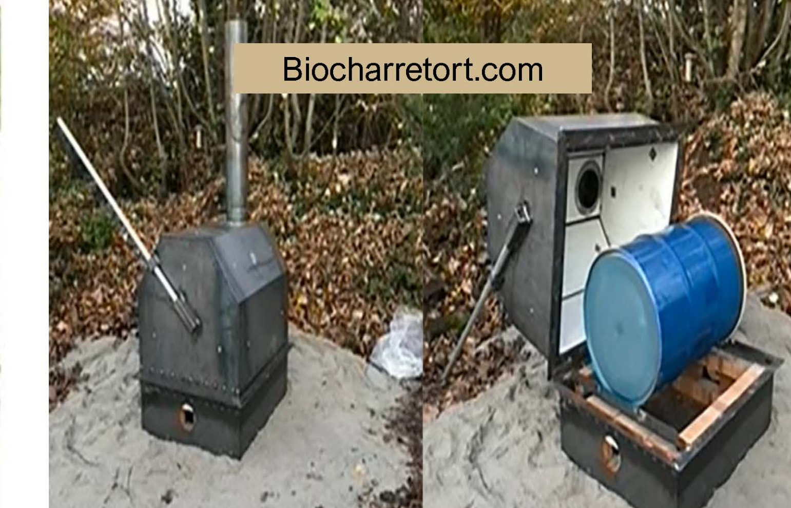
Figure 13. The Dartmoor Dragon Retort: good for biochar and can be designed for charcoal
