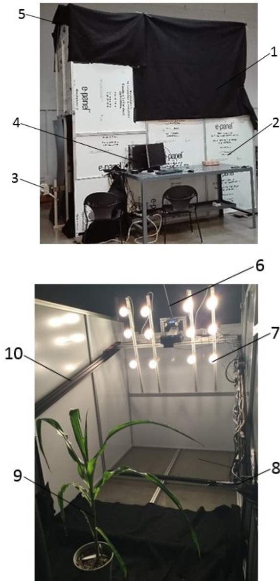
Fig. 2.1. Structure of the swing hyperspectral imaging tower: outside and inside settings
