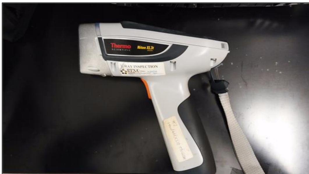
Figure 1 XL3t GOLDD+ portable XRF device from Thermo Fisher Scientific
