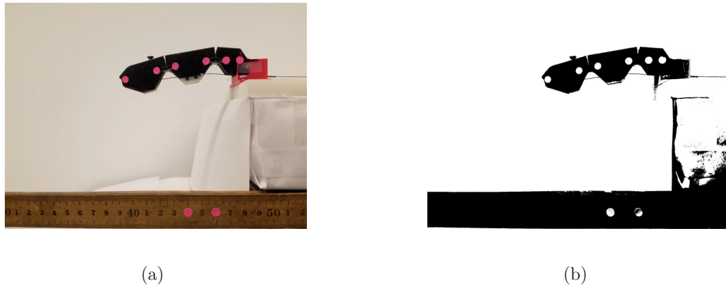
Fig. E.2. Example of Conversion Process (a)Original image (b)Binary image of the red color space.
