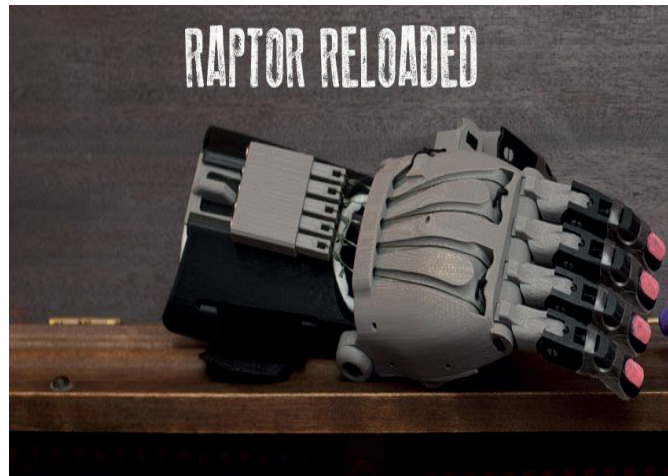
Fig. 1.4. Wrist operated 3-D printed prosthetic hand [9].
