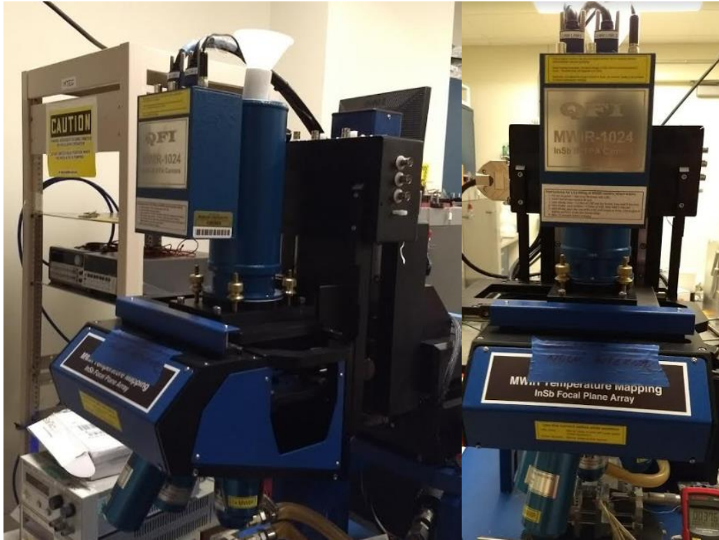
Figure 4.12 The QFI Infrascopie IR Microscope
