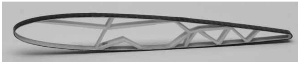
Figure 2.4. Compliant airfoil using a belt-rib concept developed by Hasse, Zuest, and Campanile in 2010 [9].
