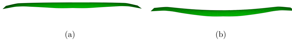
Figure 3.7. Results of Abaqus analysis showing stable states of (a) prestrained structure and (b) buckled structure for 0.3 % prestrain.
