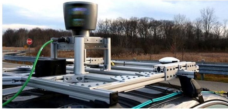
Figure 1.7 Conventional LiDAR spinning on the roof of a vehicle [11]
