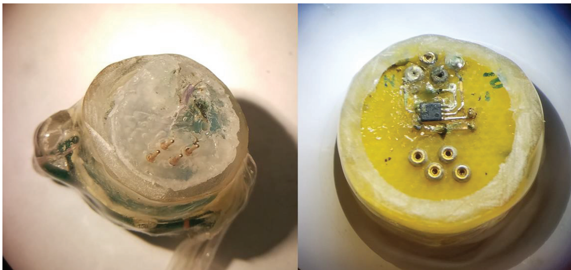
Figure 2.16 Explanted and disassembled Bionode device. Top (left) has been removed with silicon and pins in place. Bottom (right) contains working device and can be repopulated with new electrodes, re-sealed, and re-implanted.
