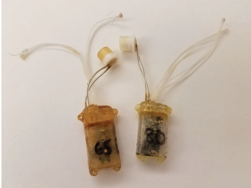
Figure 2.17 Bionode devices after sterilization cycles in an autoclave. Device on the left remained fully functional after ten standard cycles (20 psi, 250° F, 20 minutes). Device on the right remained fully functional after one increased intensity cycle (30 psi, 270° F, 20 minutes).
