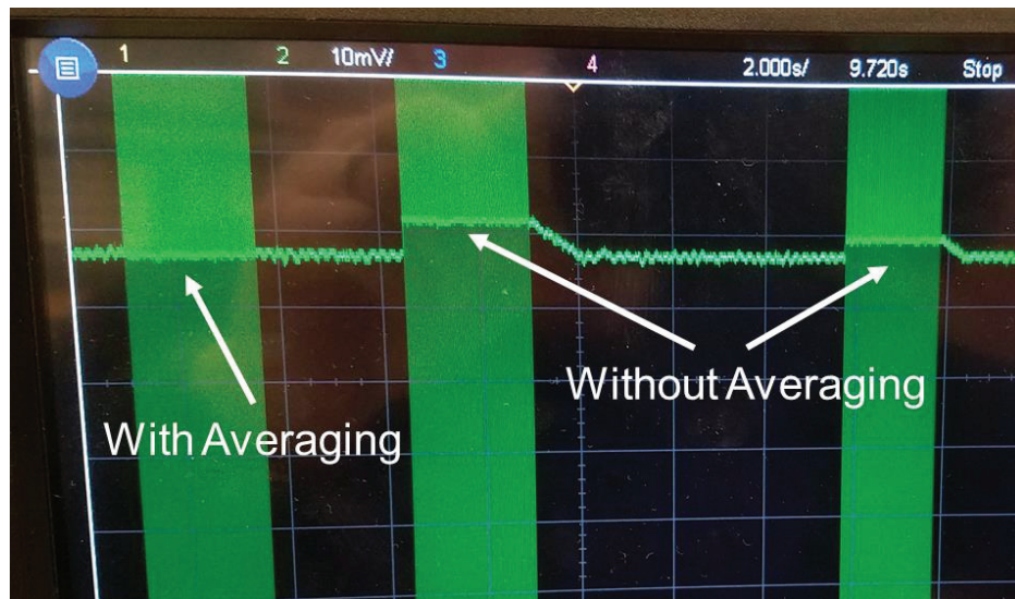
Figure 2.8 Oscilloscope image of DAC stimulation outputs (which appear as solid green sections) with and without hysteresis averaging.
