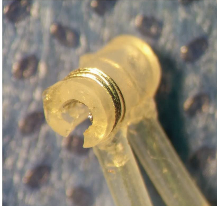
Figure 4.2 Photograph showing a standard stimulation cuff used in our studies. Threaded wire electrode was used as a grounding reference for stimulation and oriented cranially.
