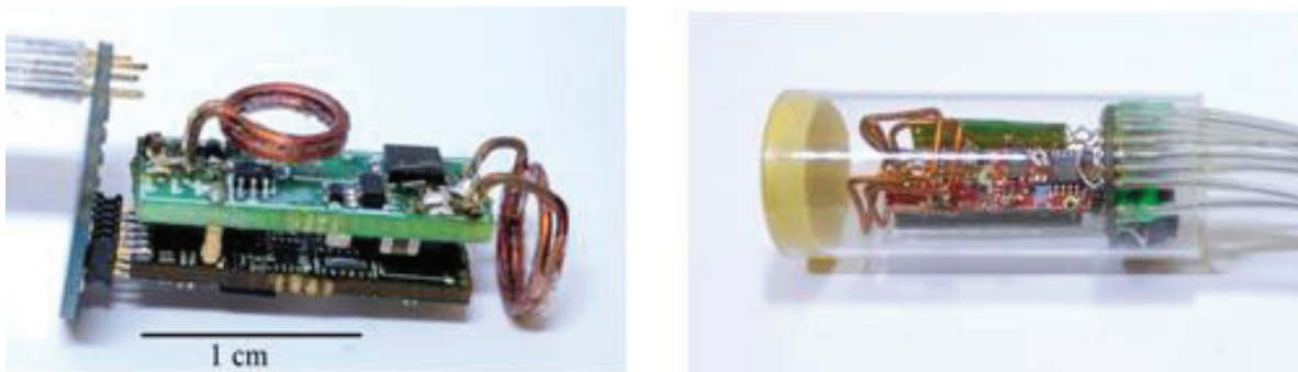
Figure 2.1 Bionode implant assembly (left) and Bionode inside glass packaging (right).
