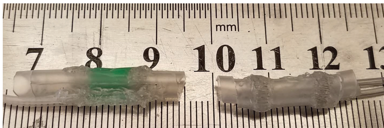
Figure 5.1 Stimulation and recording cuffs for cervical vagus nerve of pig. Cuffs each featured two electrodes made of horizontally threaded PtIr wire surrounding the inner cuff circumference. Edges of cuffs were cut in a spiral to improve stability on the vagus nerve.
