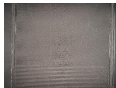
Figure 3.25. Test run 2E; higher pressure drop measured (2014).
