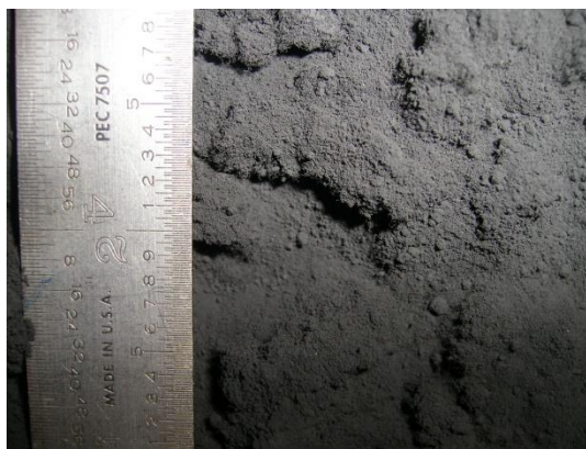
Figure 3.39. Test dust sample with clumps.
