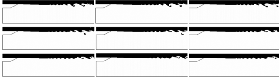
Figure 2.5.: Time steps from axisymmetric simulation showing effects of liquid turbulence mechanism. Turbulent eddies roughen the film, creating undulations that eventually grow large enough to break into droplets [41].
