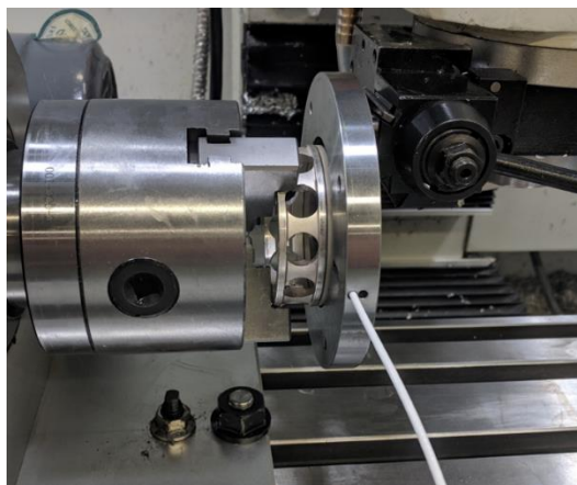
Figure 5.7. Cage rotation measurement setup on a CNC machine.
