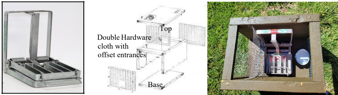
Figure 2. (L) DOC 250 trap. (R) DOC 250 trap exclusionary box diagram and complete set with the top open, showing the two offset entrances through hardware cloth (to the left of trap) to prevent non-target capture.
