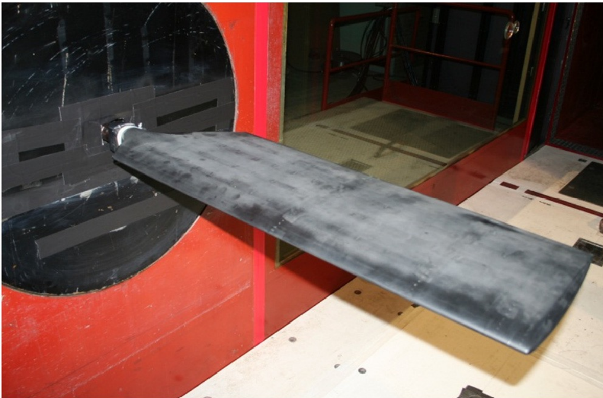
Figure 3.2: Finite OA209 wing (C300-3D model) mounted in the ONERA F2 wind tunnel (from Ref. [23])
