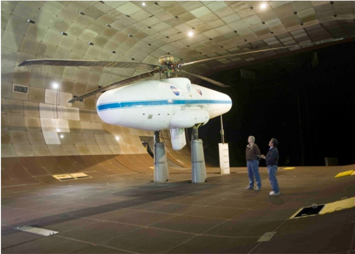
Figure 3.7: UH-60A rotor mounted on the LRTA in the NFAC 40-by-80 ft. wind tunnel at NASA Ames Research Center in Moffett Field, California (from Ref. [30])
