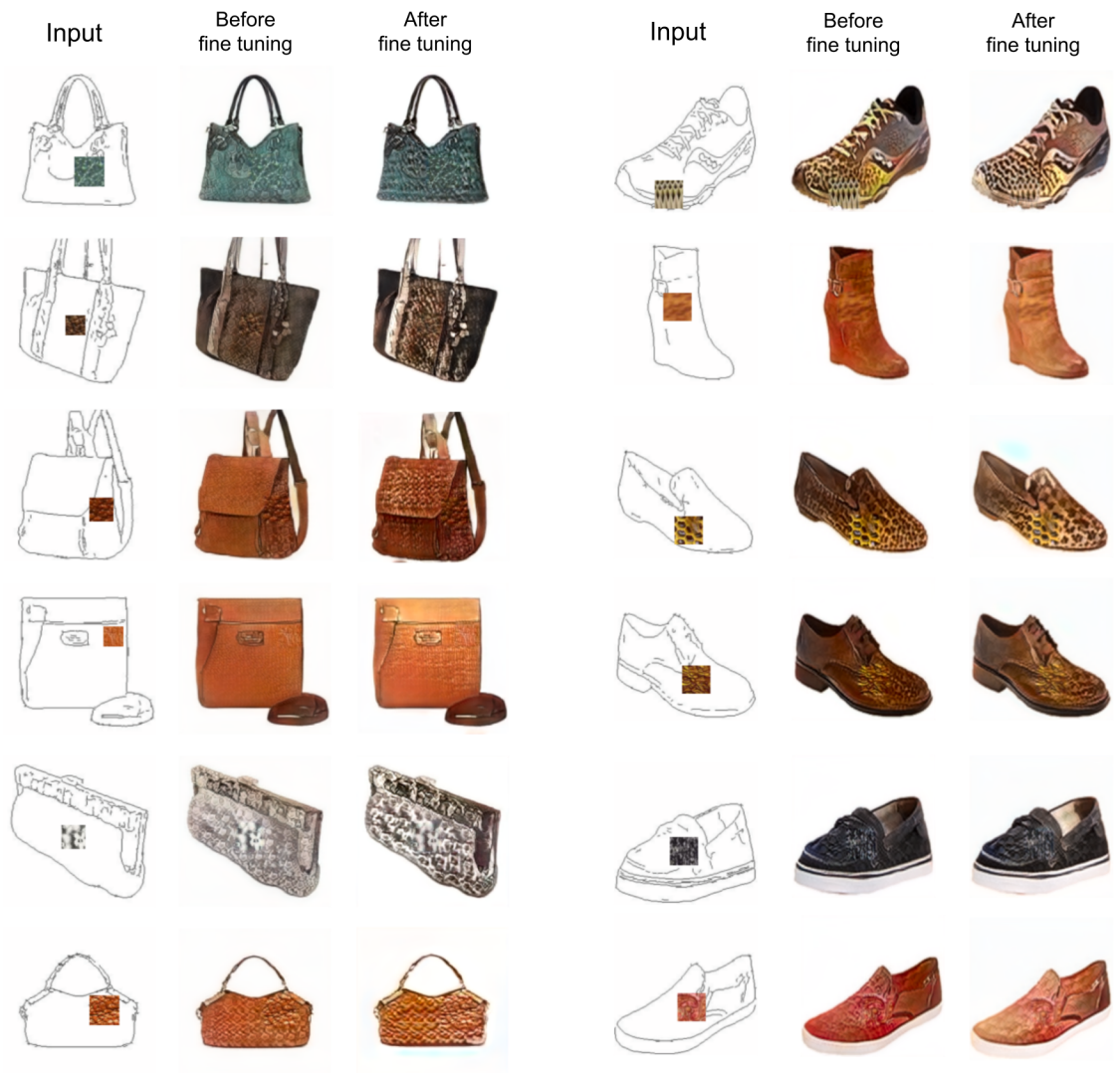
Figure D.4: Comparison of results before and after fine-tuning on an external texture database. The base model is trained on handbag and shoe sketches with ground truth images. The fine-tuned model with local texture loss improves texture propagation on difficult texture with high contrast and strong regularity, e.g. striped, dotted, checkerboard patterns, which are rarely seen in the ground-truth.
