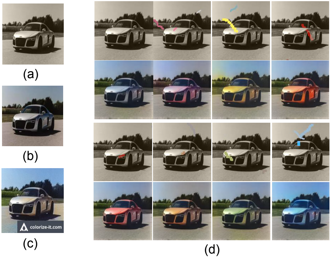
Figure 3.8: Guided Image Colorization: a) grayscale input, b) original color image, c) deep colorization result [114], d) First and third rows: color strokes overlaid on top of the grayscale input (zoom in to see the color strokes). Second and fourth rows: colorization results.
