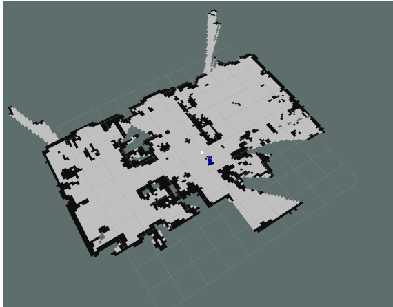
Figure 8.6: A map of the ESM G13 room in the AE department, Georgia Tech, generated using the Hector-SLAM algorithm on the RACECAR robot.
