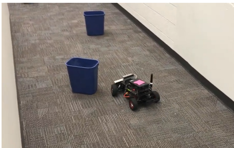
Figure 8.7: Running the obstacle avoidance module on RACECAR hardware
