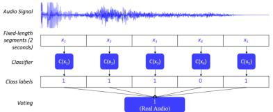
Figure 5: Segmenting the data to feed into the classifier and using the max count as the final prediction
