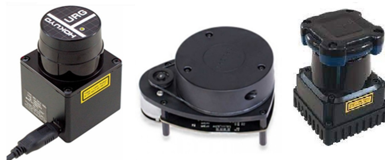
Fig 1. 2D Laser scanners (left) URG-04LX (middle) RPLidar A1 (right) UTM-30LX.
