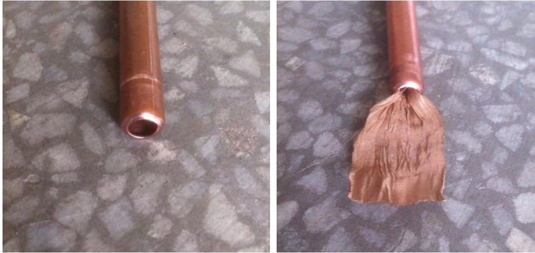
Fig. 2. Inner structure of the two different types of heat pipe (a) wickless heat pipe (b) wire-meshed heat pipe.
