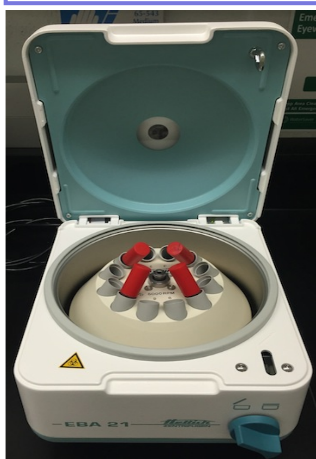
Fig. 5: EBA 21 Hettich Zentrifugen was used for separating the supernatant from the pellet at 5,000 rpm for 5 minutes.
