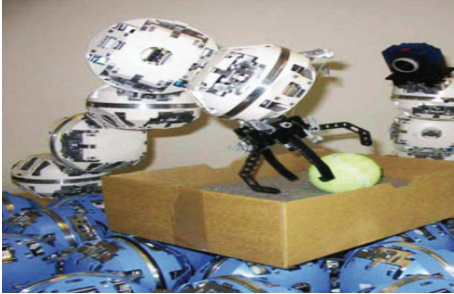
FIGURE 1: Lattice type architecture [20] (copyright @ 2007 Brandt et al.).
