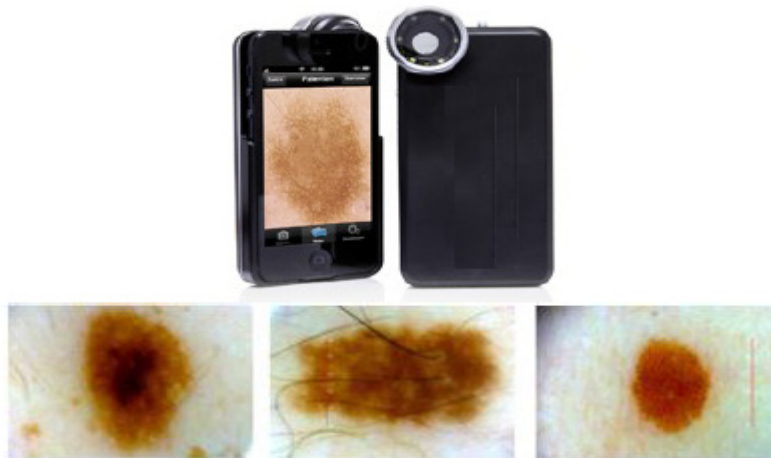
Figure 9. The dermatoscope device attached to the iPhone and sample of images captured using the device
