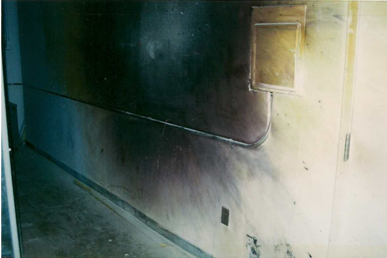
Figure 2: Steel and steel vaporized on to wall (black and purple). Copper (orange) vaporized on to wall also.
