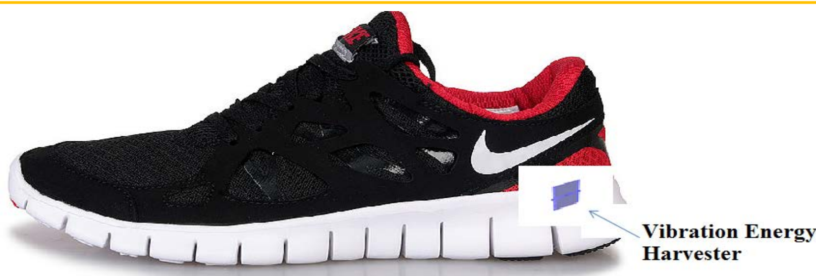
Figure 1. Shoe with vibration energy harvester inserted in its sole
