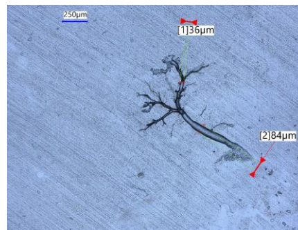
Fig. 4. Electrical track within epoxy resin formed between 60 and 85 hours.
