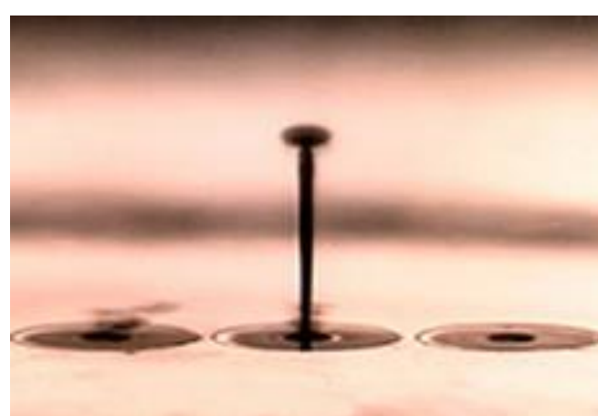
Figure .1 Droplet of Inkjet impact on paper
