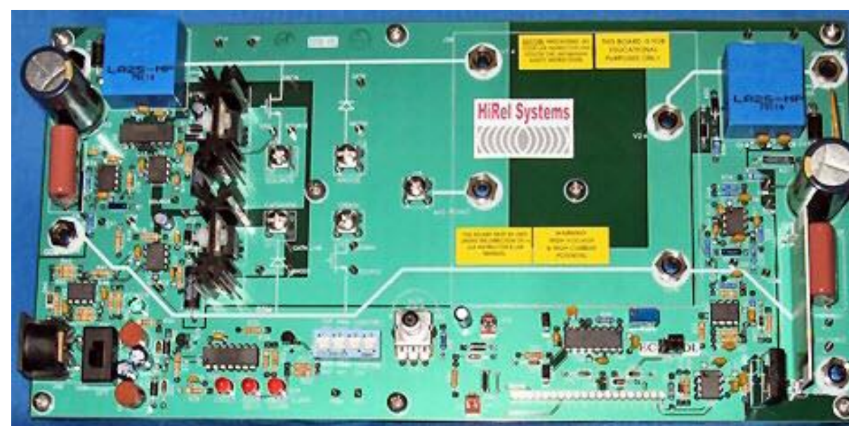
Figure 2: power pole board
