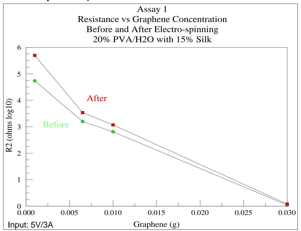
The green line represents resistance across the comb circuit before electrospinning, the red line after electro-spinning. It is clear that resistance across the comb circuit drops as graphene concentration on the circuit surface increases providing additional evidence of graphene as a soft conductor. Also, it shows that resistance increases after electro-spinning fibers onto the comb circuit providing evidence that the fibers act as a resistor.
