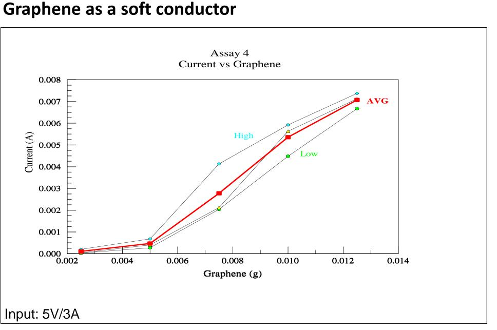
This graph shows the relationship of conductivity to graphene concentration on the comb circuit for Assay 4 which consisted of 15 printed circuit boards. 5 different graphene concentrations were used with 3 circuit boards per concentration. It is clear that conductivity rises as graphene concentration increases on the circuit surface. The green line indicates low range, the yellow mid-range and the blue high range. The red line is an average of the three.
