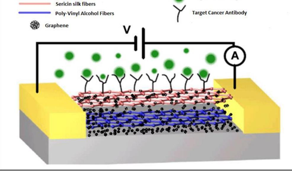
Conductive graphene allows current to flow between comb circuit electrodes. Electrospun poly-vinyl alcohol and Sericin silk create sticky foundation for attachment of target cancer antibodies. Target cancer antigens spontaneously bind with antibodies and change the potential and impedance of the circuit
