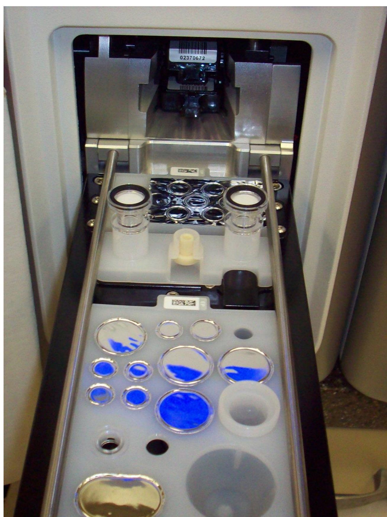
Figure 3. Verigene Processor SP drawer assembly. Pictured from top to bottom is the test cartridge, amplification tray, tip holder assembly, and extraction tray.
