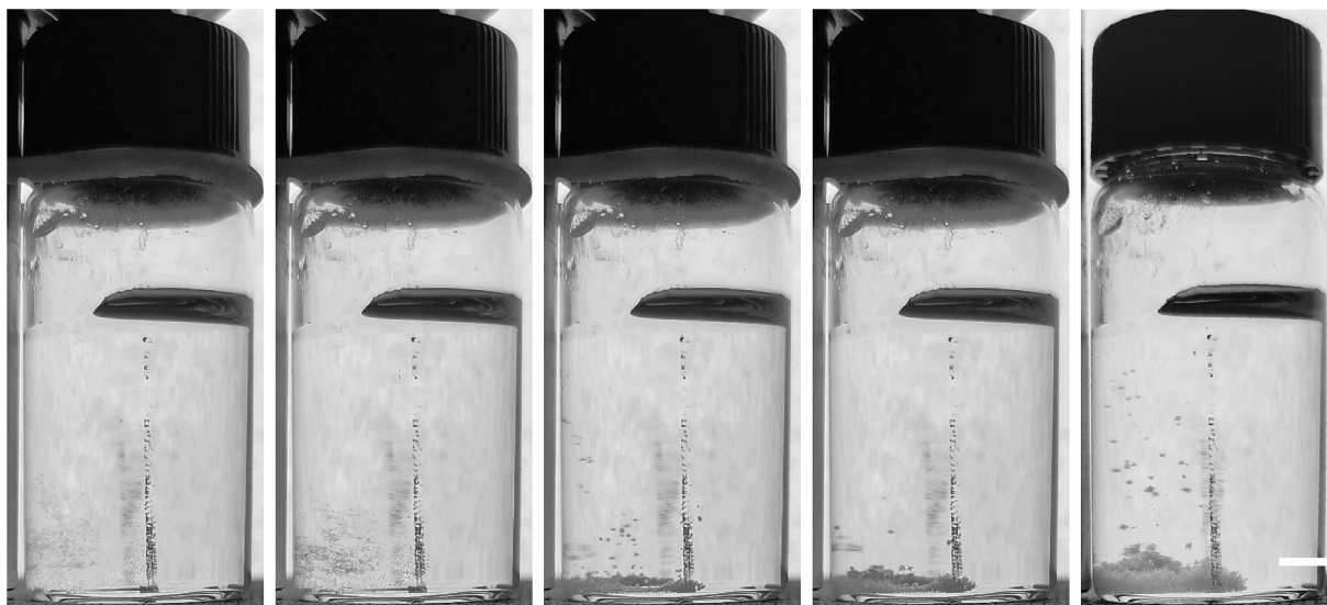
Fig. 7. Sequence of images demonstrating MSIN of \text{NH}_4\text{Cl} crystals. The scale bar represents 5 mm. See video S2 in the Supporting Information. The left half of the inner surface of the vial has been treated with a hydrophobic coating. The right half has been left untreated; the vertical boundary has been marked with a pen. The deformed liquid meniscus demonstrates the water repellent feature of the coating. The solution was aqueous supersaturated \text{NH}_4\text{Cl} ( C = 8.88 \text{ mol kg}^{-1} , S = 1.09 , 35^\circ\text{C} ). The vial was struck with a block of mass m = 200 \text{ g} from a height d = 10 \text{ cm} , using a soft floor as base. Images from left to right: 2 s, 3 s, 10 s, 20 s and 60 s after impact. It can be seen that the solid nucleates exclusively in the hydrophobic half of the vial. After 10 s (third panel) the crystals have sedimented to the bottom. By 60 s there is evidence of secondary nucleation coupled with internal fluid flow.
