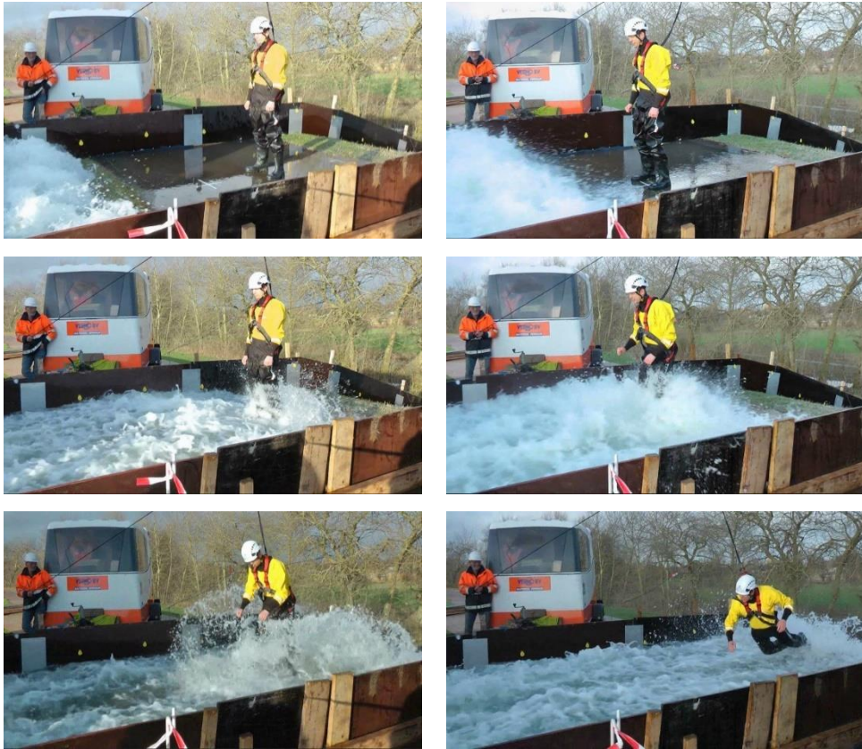
Figure 16: A wave overtopping volume of 1500 l/m passing the crest (left pictures). The feet slipped away about 0.2 m. A wave overtopping volume of 3500 l/m passing the crest (right pictures). The volunteer was washed away.
