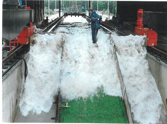
Figure 2: Test 114 in the Delta flume with q = 10 l/s per m. The person was stable during the whole test of 1.5 hours. Picture taken from Smith (1994).
