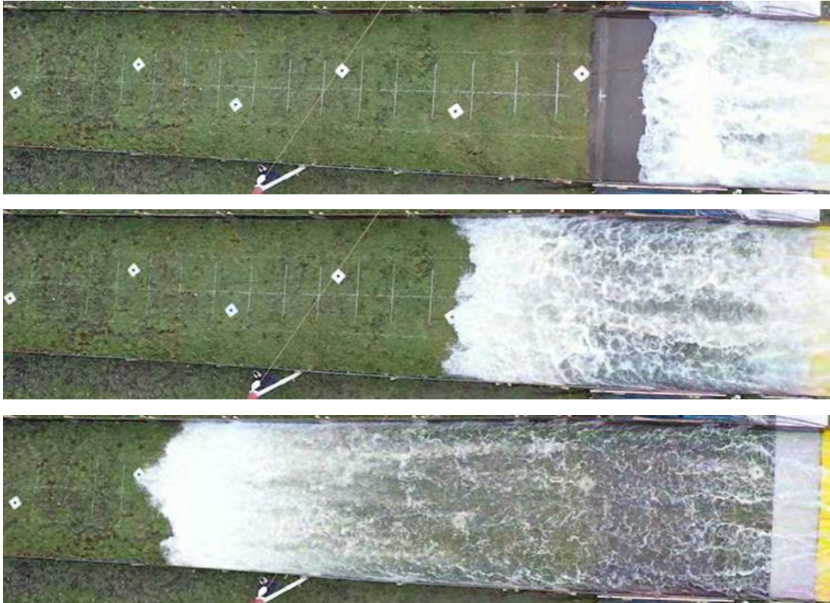
Figure 10: Irregularity of the overtopping wave front. Above: at the middle of the crest (4 m); middle: at paddle wheel 3 (8.5 m); below: at paddle wheel 6 (17.5 m). Overtopping wave volume of 1500 l/m.
