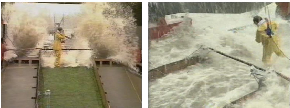
Figure 3: Test 112a in the Delta flume with q = about 25 l/s per m. Left: a wave breaks onto the 1:4 slope and a person is standing on the crest attached to a life line. Right: one of the occasions that the volunteer became unstable and was saved by the life line. Pictures are taken from the video of this test.
