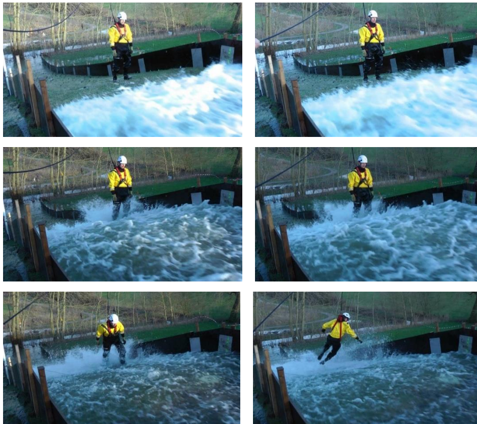
Figure 17: A wave overtopping volume of 1250 l/m passing the slope (left pictures). The volunteer stepped back about 0.5 m. A wave overtopping volume of 2000 l/m passing the slope (right pictures). The volunteer was washed away.
