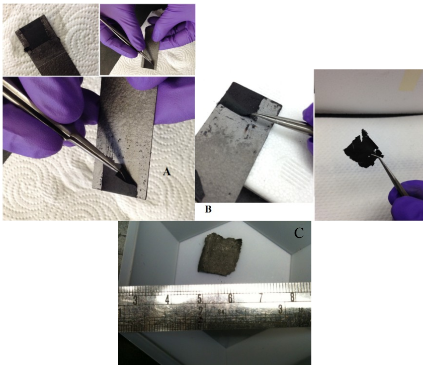
Figure 5-3: Optical images of PPy film formation on graphite substrate. A free standing film can be peeled off to be used as an electrode. A) Control PPy film, B & C) PPy-graphene-CNT film.
