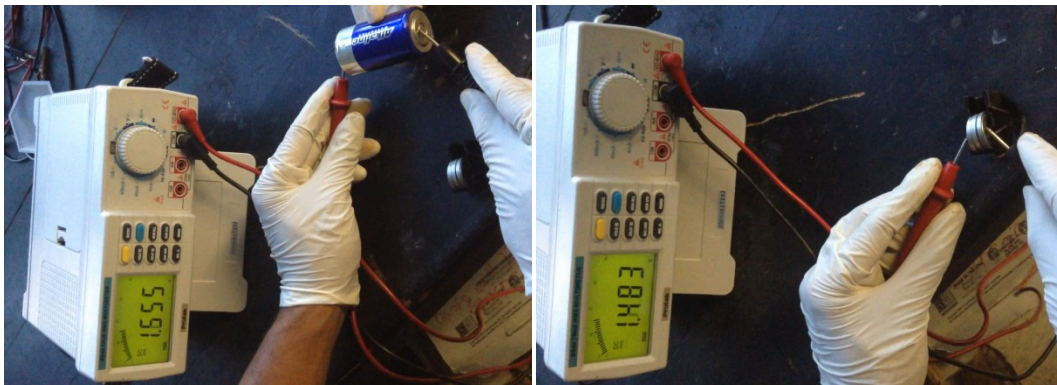
Figure 6-5: A) Supercapacitor device assembled and ready to be tested. B) Measurement of the output voltage from a conventional alkaline 1.5 V battery, C) Output voltage of supercapacitors stacked in three cells made from CR2032 stainless steel coins. The overall output voltage of the device is approximately 1.5 V
