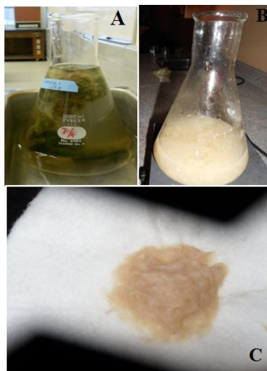
Figure 4-1: A) Optical image of algae ball prior to cellulose extraction, B) Algae cellulose extracted in pulp form after the hydrolysis, C) Filtered cellulose pulp
