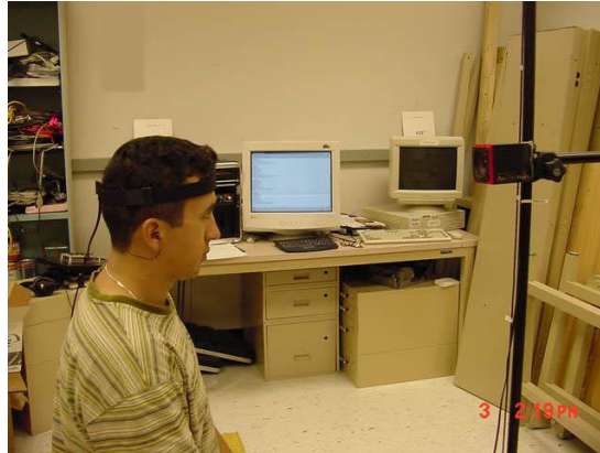
Figure 1. Measurement of HRTFs using Ausim3D's HeadZap System
