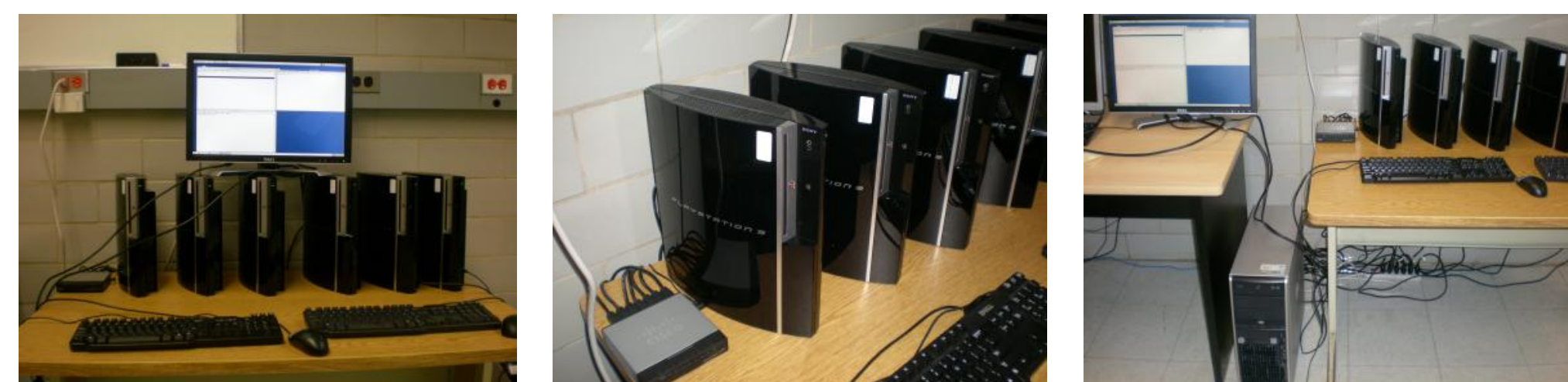
Fig. 2 Pictures for implemented PS3 Cluster
