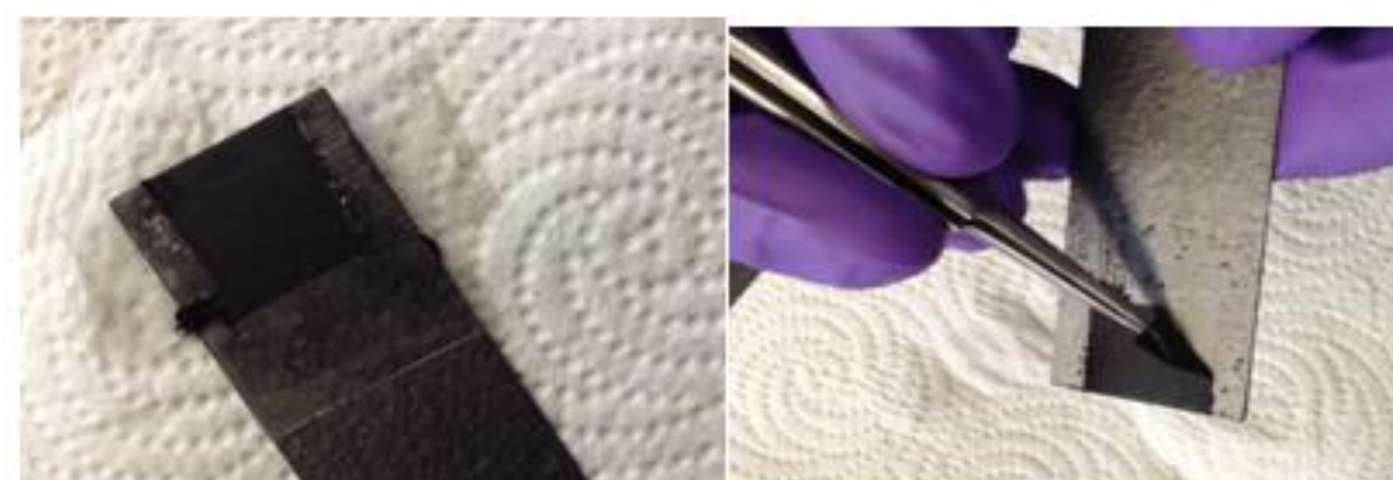
[A, B] Images of the PPy film made using electrodeposition method, [C] Scheme showing the electrodeposition method, [D, E] images of the PPy-graphene film using electrodeposition method
