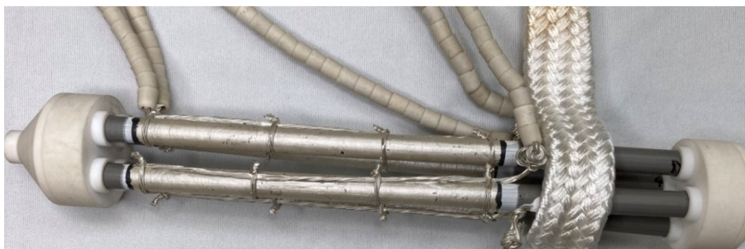
Figure 8.40 - 4 cell stack with hiTRAN-only current collection.
