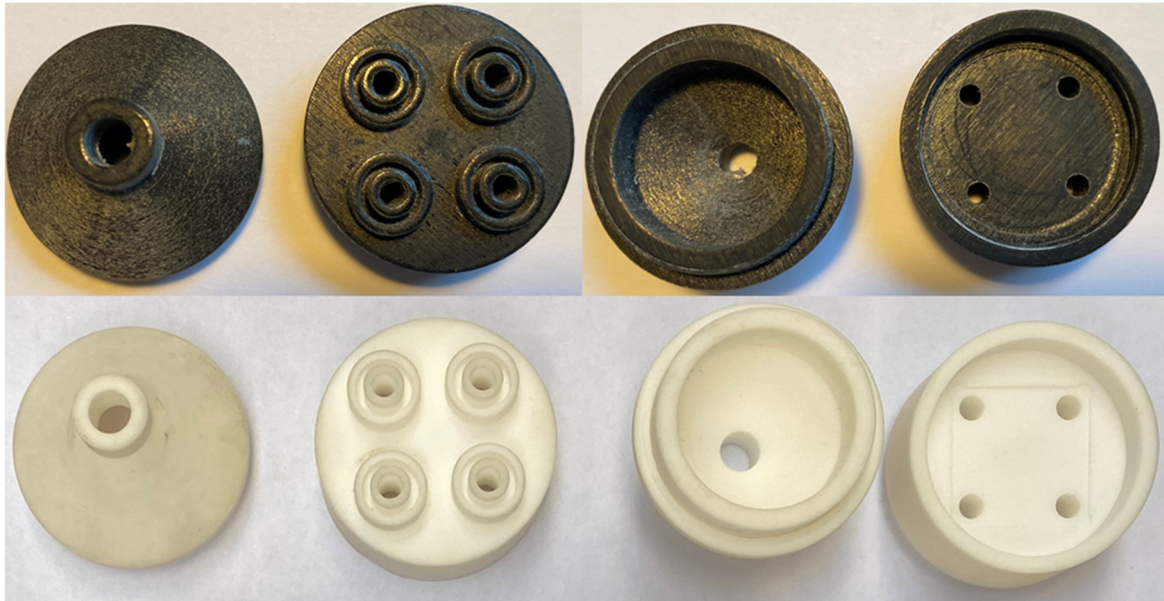
Figure 8.36 - 3D printed (plastic) and machined Macor 4-cell stack manifolds.
