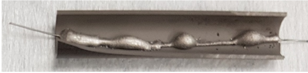
Figure 7.8 - Anode stub and nickel wire brazed with BNi-9 showing braze pooling.
