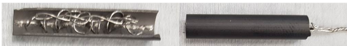
Figure 7.9 - Continuous brazed fuel cell stubs using BNi-2 braze to join hiTRAN to the anode.
