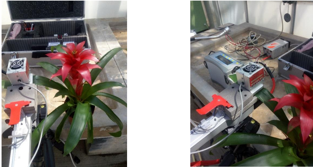
Figure 3-1: Images of the experimental setup for leaf CO 2 assimilation measurements, equipment pictured includes infra-red gas analyser, leaf cuvette and external halogen light source.
