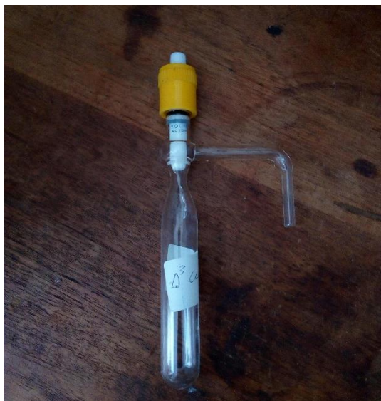
Figure 6-2: The cold finger used for experiments containing pure alpha-pinene standard.
