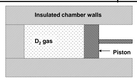
Dense gas of D<sub>2</sub> undergoes adiabatic compression Rapid process - - explosively driven Well-insulated chamber – retain energy internally
