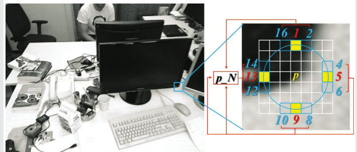
Figure 2: The ORB feature extraction process of the OG-SLAM framework. P_N represents the neighbor pixel, N corresponds to its index. OG-SLAM only calculates the illumination difference between p and the yellow pixels ( N_1, N_5, N_9, and N_{13} ). (a) represents a certain image from the dataset. (b) is the pixel layout around pixel p .
