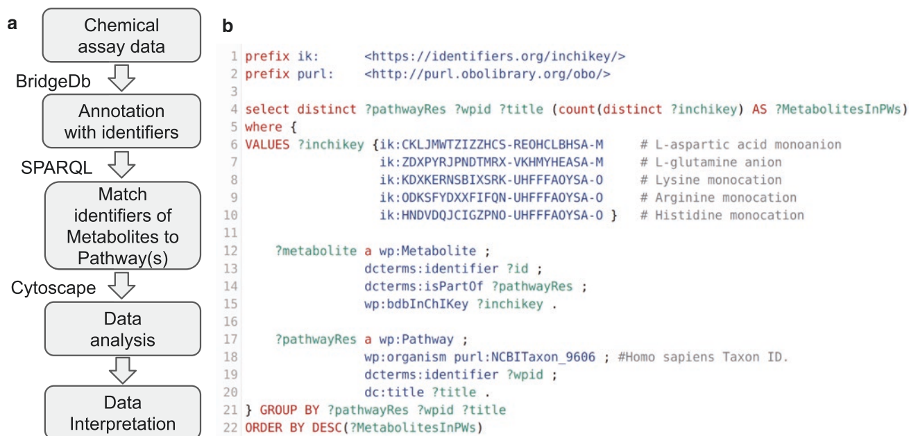
Fig. 73.6 Proposed workflow for data analysis of metabolic biomarkers with semantic web technologies. (a) Moving from chemical assay data to data interpretation using BridgeDb, SPARQL and Cytoscape. (b) Example of a SPARQL query on metabolic data in the WikiPathways RDF
